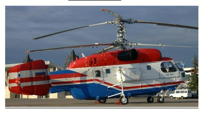
The Kamov Ka-32A is an autonomous high-power-to-weight-ratio compact air transporter that can operate independently of ground support. The main roles of the Ka-32A civil helicopter are as passenger and cargo transport, a flying crane for building construction, transport for bulky cargo up to 5t carried on an external sling, logging, search and rescue, medical and emergency evacuation, loading and unloading ships at sea and offshore operations.
